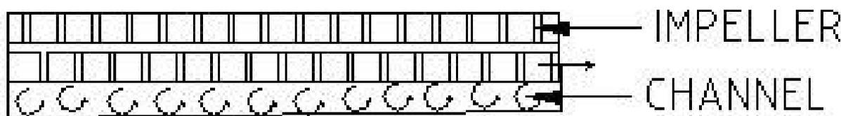
Fig 5 Tapered channel to improve efficiency of Regen pump
