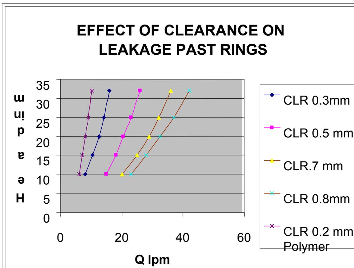
Fig6 Effect of Clearances on Leakage Past Wear Ring
