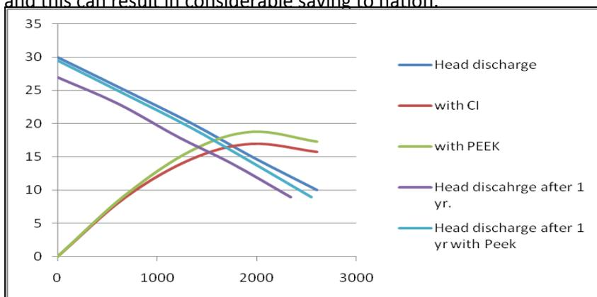
Fig 4 Improvement in efficiency with PEEK.
