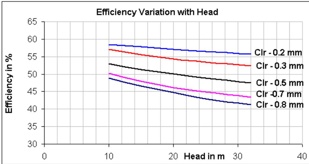
Fig 7 Efficiency variations for a duty point discharge of 80 lpm for various clearances
